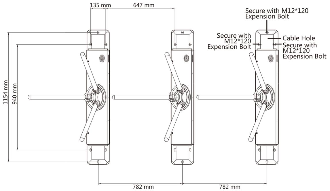
**Figure 3-3 Installation Footprint**
