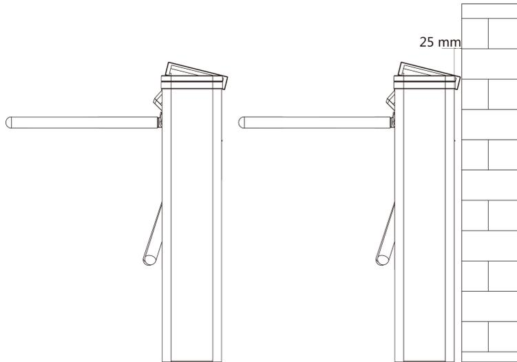
Face recognition terminal installed: If the installation area is too close to the wall, make sure the distance between the pedestal and the wall should be more than 130 mm, or the surface may be scratched.
